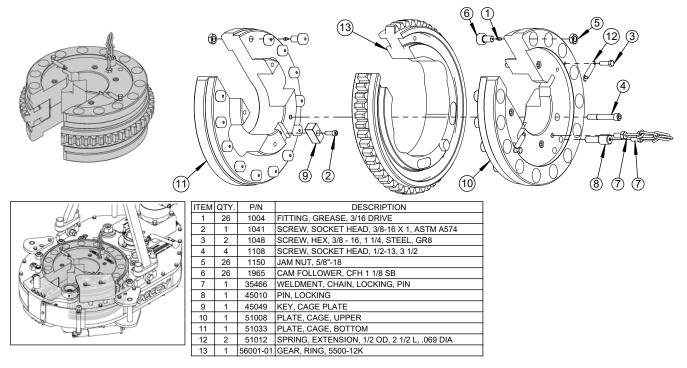
Illustration 7.4: 51080 ASSEMBLY, CAGE PLATE, RING GEAR
