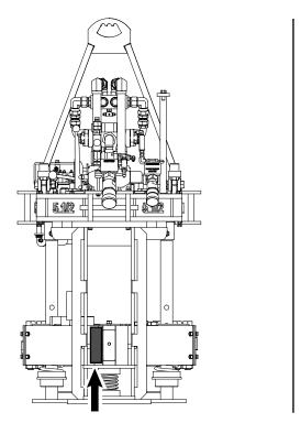
Illustration 3.5.2: Make Up Load Cell Configuration
