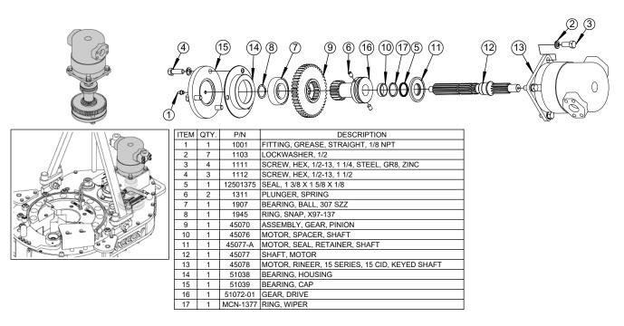
Illustration 7.5: 51081 ASSEMBLY, MOTOR, DRIVE GEAR
