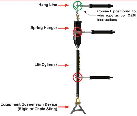
Illustration 3.2.1: Correct Installation of Positioning System
